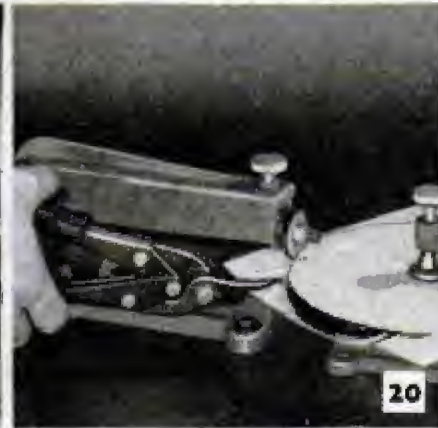
Circles are cut by using a pivot, which is an accessory to the shear. Cut may be started at edge of work, as in bandsawing, or top cutter can be forced through work at any point. To prevent distortion, inside cuts are made with minimum overlap of the cutters. On outside cuts, snip away the waste as cut progresses
